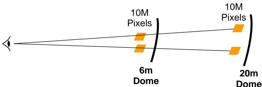
Typically the human eye can perceive a spatial resolution between two adjacent pixels of 3 arc minutes ( $3 \times 1/60^{\text{th}}$  of a degree). Higher resolution is perceivable but typically only if there is a visible reference point available (i.e. comparing 3 arc minutes with 1 arc minute on screen).
