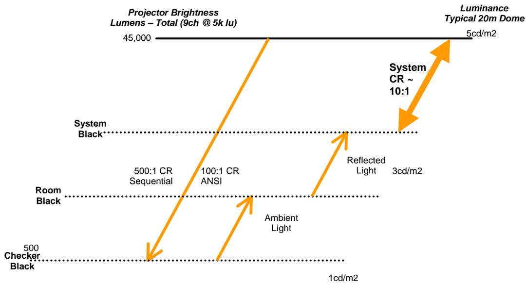
With checkerboard content displayed in a hemisphere, expect to measure around 10:1 CR.
